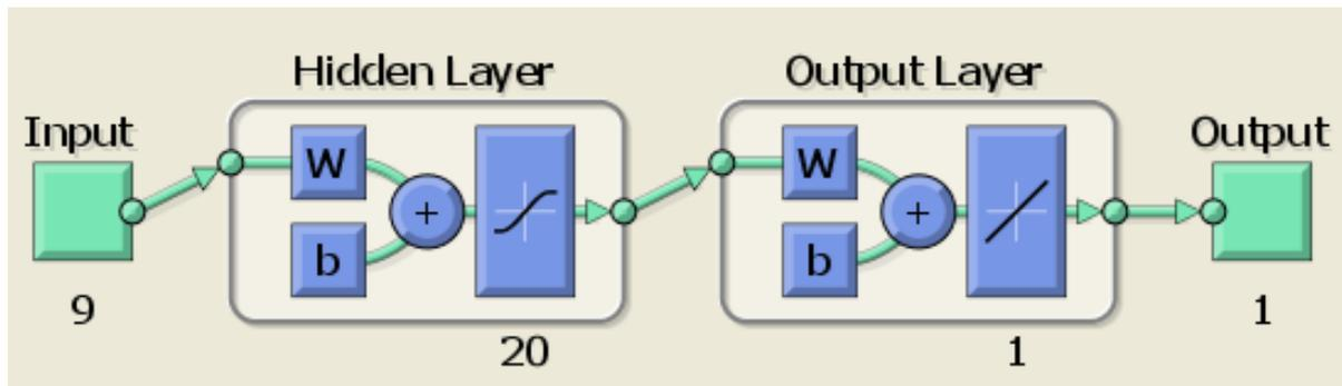
**Figure 3** The neural network structure for weight estimation of camels based on digital images features
