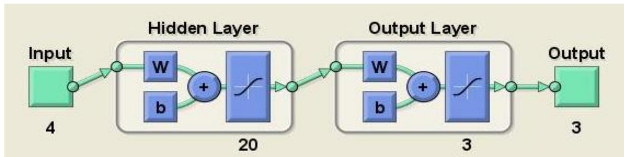
**Figure 7** The ANNs structure for pelt color classification
